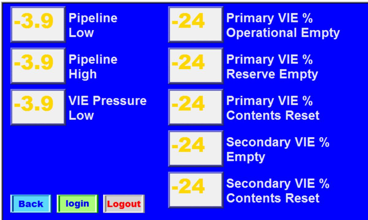
At the bottom left are three buttons, the blue “back” button takes you to the main display page, the green “login” button takes you to the login page (you will need to login before any alterations can be made to the settings page, instructions on how to login are in section 3 later in these instructions) and the grey “logout” button to prevent unauthorised change of the settings.
